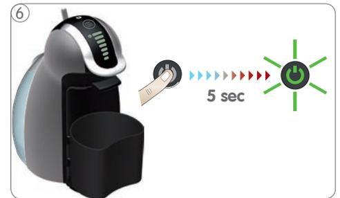
⑥ Press and hold power button for at least 5 seconds. Power button starts blinking green and machine enters the descaling mode.
