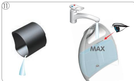
Empty capsule bin. Fill water tank with fresh, drinking water up to max. level.
