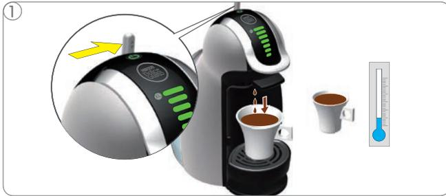
① If the beverage only comes out in droplets or if the beverage is cooler than usual, the machine has to be descaled.
