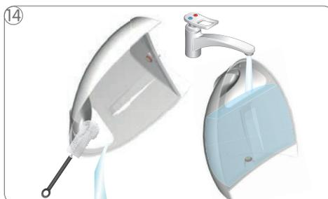
Rinse and clean water tank. Afterwards refill with fresh, drinking water and insert it to machine.
