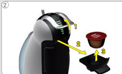
Lift the locking handle and remove the capsule holder.
