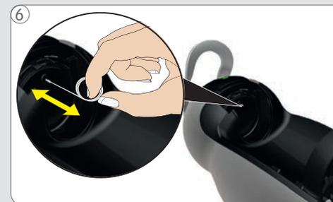
Unblock the injector with the cleaning needle.
