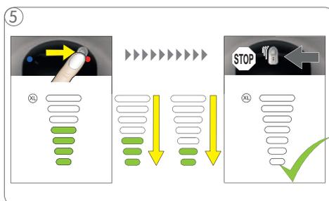
Move the lever to the right for hot beverages and to the left for cold beverages. Beverage preparation starts. Bar display lights vanish progressively. Machine stops preparation automatically. Extraction can be stopped manually by moving the lever back to the middle position.
