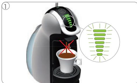
① Error symptoms: Beverage preparation stops part way during delivery or does not start at all. Bar display flashes and power button blinks red and green rapidly.
