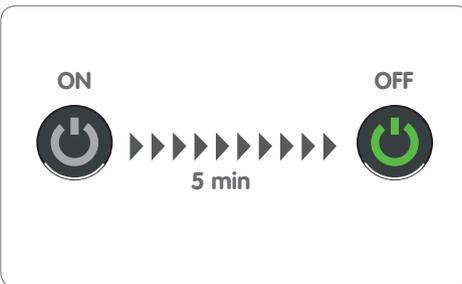
After 5 minutes of non-usage the machine automatically shuts down (Economy Mode). To restart, press power button.
