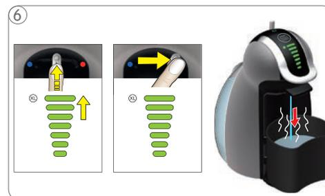
6 Rinse the machine as follows: Light up all bars to max. level using the lever and then move it to the right. Machine starts rinsing. Lights on the bar display vanish progressively.
