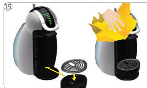
Place drip grid on drip tray. Then insert drip tray at desired position of machine. Clean machine with a soft damp cloth. Dry it afterwards with a soft dry cloth.
