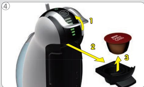
④ Then lift the locking handle and remove the capsule holder.
