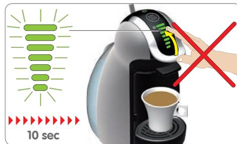
⚠ After finishing preparation the bar display flashes and the power button blinks red for about 10 seconds. **During this time do not open locking handle!**
