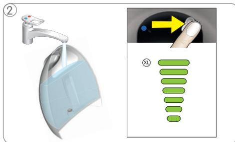
② Check if there is water in the water tank: if not, refill and press hot/cold button again to continue preparation; if the water tank is full proceed as follows:
