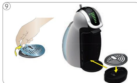
9 Remove protection foil from drip grid. Place drip grid on drip tray. Then attach drip tray at desired position on machine.
