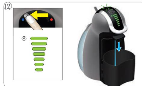
Move lever to the left for cold extraction. Bar display begins to count down. At end of rinsing cycle power button lights up red and bar display counts up.
