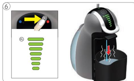
6 Continue rinsing with hot water: Push the lever up to set the bar display to maximum level. Move lever to the right for hot extraction.
