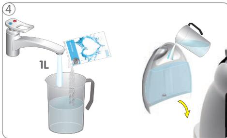
④ Mix 1 litre fresh, drinking water with descaler sachet in a measuring cup. Pour descaling solution into water tank and insert water tank to machine.
