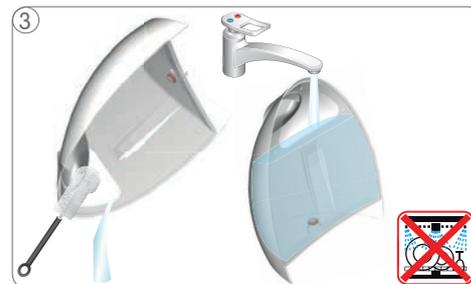
3 Rinse and clean water tank. Afterwards refill with fresh, drinking water and insert it to machine. The water tank is not dishwasher proof!
