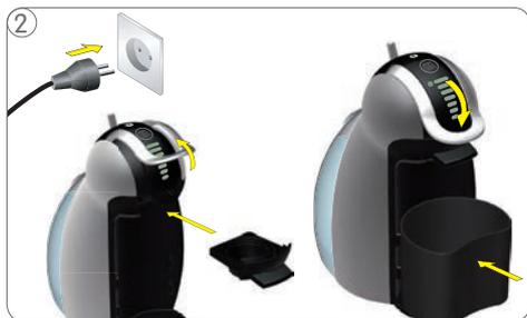
2 Open locking handle and insert empty capsule holder. Close locking handle. Place capsule bin under outlet. Connect power plug to mains power socket.
