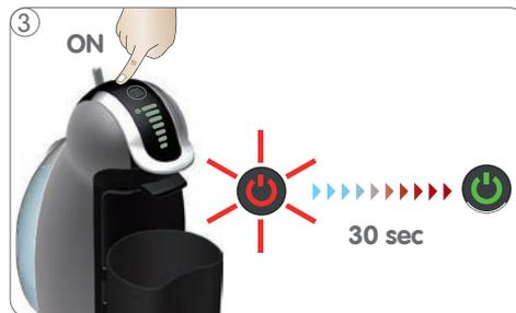
3 Switch machine on. While machine is heating up, power button starts blinking red. After approx. 30 seconds, power button lights steady green and machine is ready.
