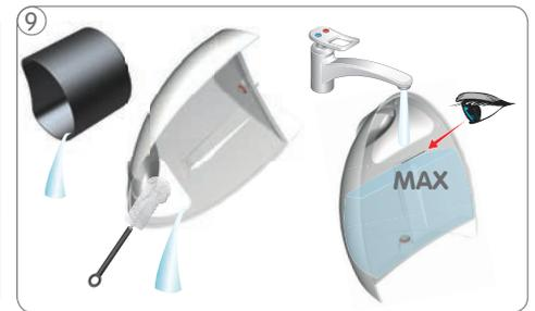
⑨ Empty capsule bin. Rinse and clean water tank thoroughly. Fill water tank with fresh, drinking water up to max. level.
