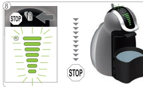
⑧ The bar display and power button are blinking green at the end of the descaling cycle.
